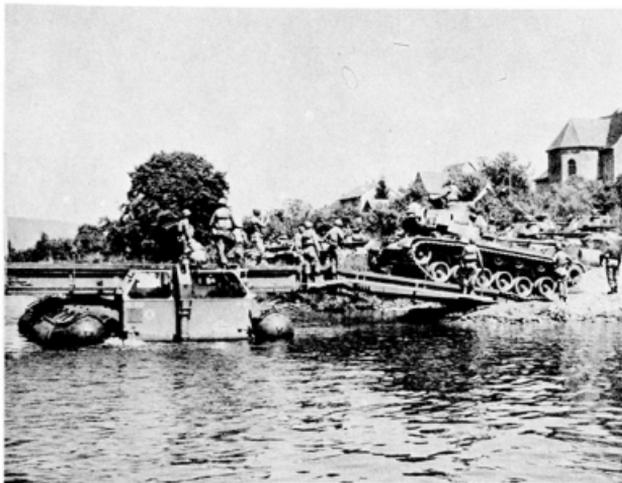
Loading of M-48 tanks on raft
